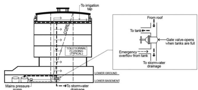
Figure 14: Rainwater harvesting system
