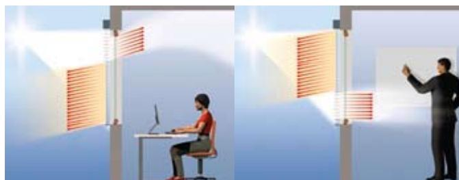
Figure 8: External automated daylight guidance blinds
