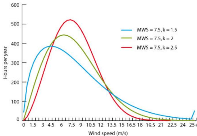
Larger values of k result in a more regular bell-shaped curve while the mean wind speed is unchanged.
