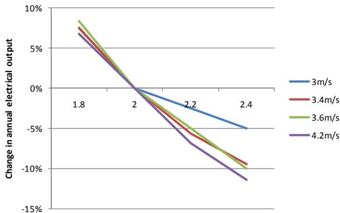
**Fig 3** The influence of Weibull shape factor on predicted electrical output from typical 12 kW wind turbine
