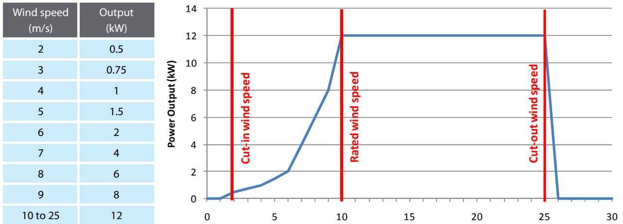
**Fig 2** Typical power curve for 12 kW wind turbine
