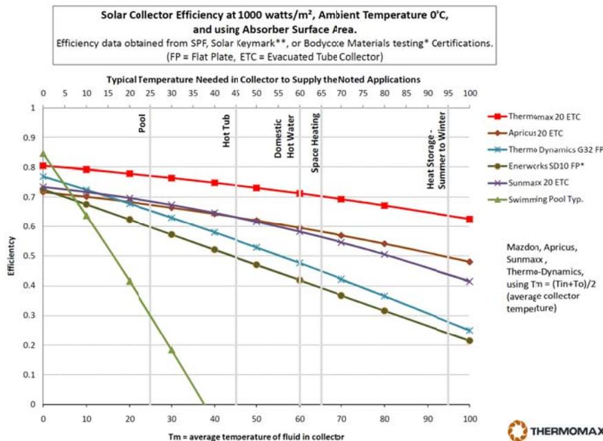
Fig 2 Measured solar collector efficiency of sample Thermomax solar systems based on aperture area (source: Thermomax Industries)
