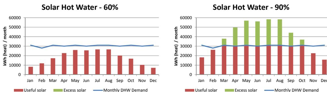
Fig 3 Monthly solar thermal energy generated compared to DHW demand
