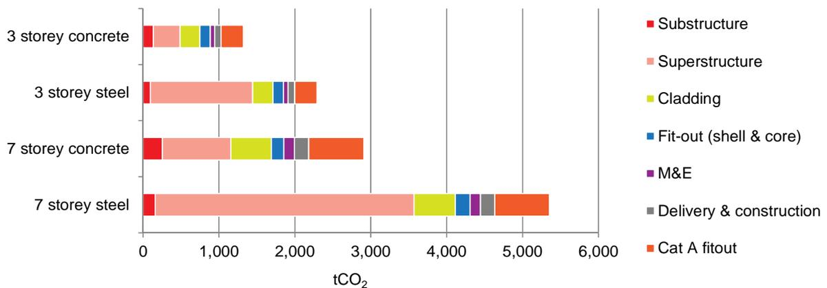
**Fig 3 Embodied carbon studies from Sustainable Concrete Architecture (source: adapted from Bennett)**
