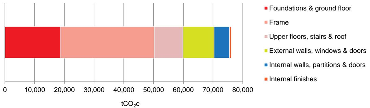
Fig 11 Leadenhall building embodied carbon breakdown (source: adapted from RICS / Davis Langdon)
