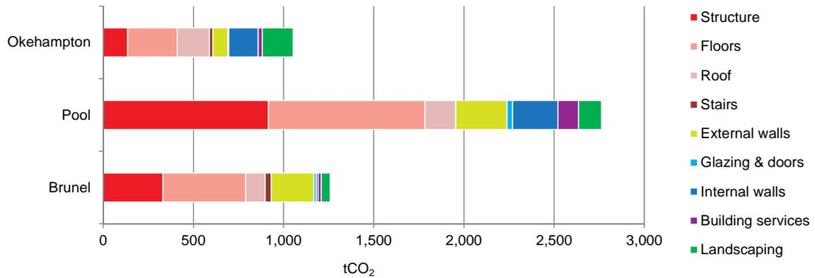
Fig 10 Embodied carbon for three regional office buildings (source: adapted from Halcrow Yolles)
